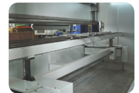
Heavy-duty 2-axis back gauge, X-R
