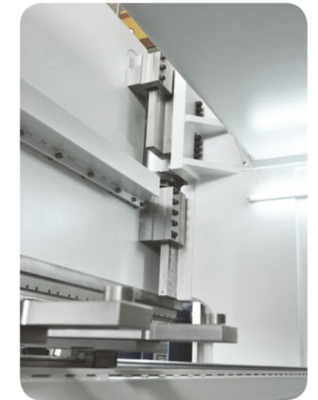
Beam movement on heavy-duty bronze sliders to secure safety and accuracy
