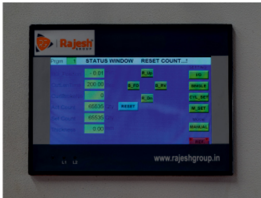
Digital touch display controller with multi step backgauge & auto angle adjustment
